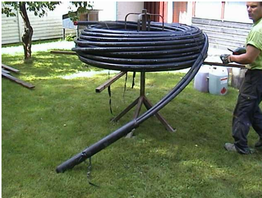
Borehole probe on a turntable to allow unwinding and insertion to the well whilst filled with water.
