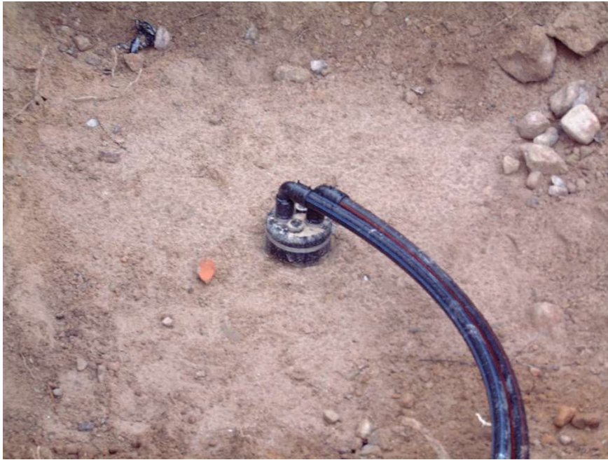
Neoprene borehole sealing cap
